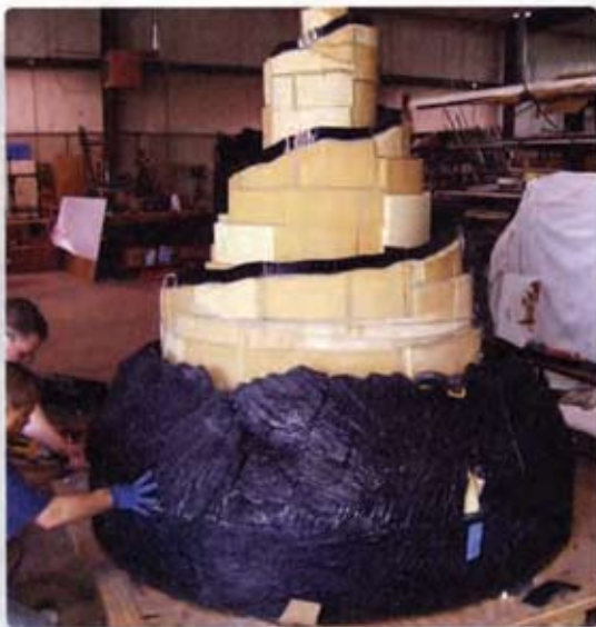
Workers covered a rigid aluminum-and-wood frame with polyurethane foam. Next, they molded semicured polyurethane casts to the structure and clamped them there. Black polyurethane glue finally bonded the casts to the structure.
