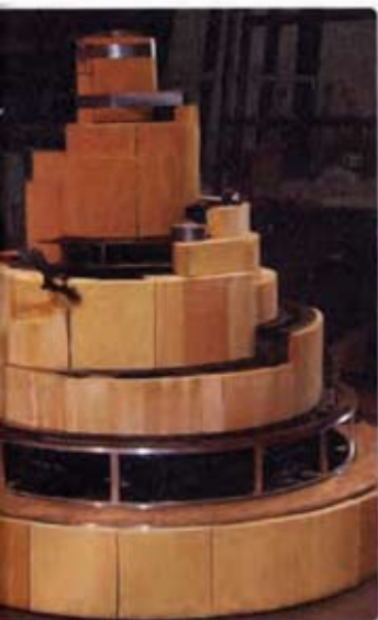
Workers covered a rigid aluminum-and-wood frame with polyurethane foam. Next, they molded semicured polyurethane casts to the structure and clamped them there. Black polyurethane glue finally bonded the casts to the structure.
